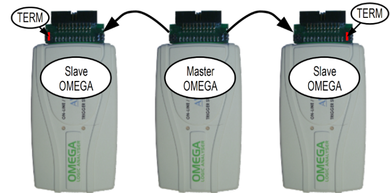
Fig. 34: Interconnection of three Logic Analyzers
