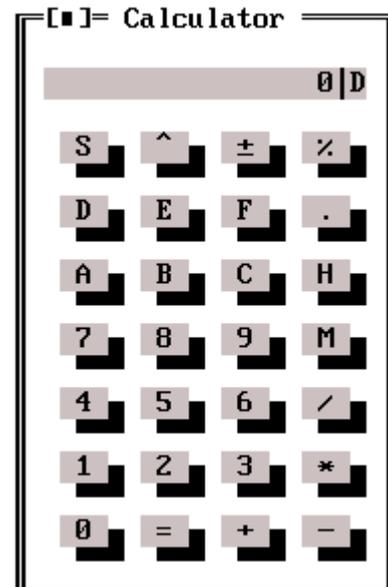
Using keys corresponding to other buttons you can enter numeric operands for calculation. Only the 0 and 1 keys in binary, 0 to 9 in decimal and 0 to 9 and A to F in hexadecimal are valid.
