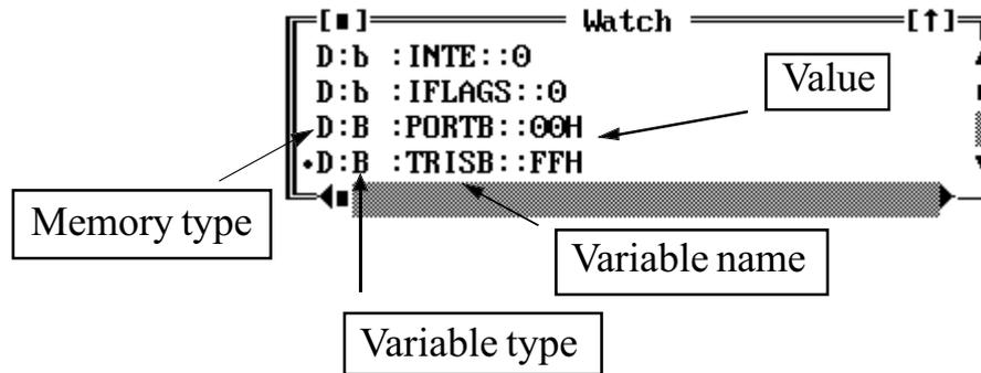
item is a register (address) value in the processor emulation memory. Four radices (hexadecimal, decimal, octal or binary) and ASCII character representation are available for displaying values. The address is always in hexadecimal. In case of bit variables, the comma character and an order of the bit (0 through 7) follows the address. In case of bit array, bits are numbered in ascending order of binary numbers as well as byte addresses.
