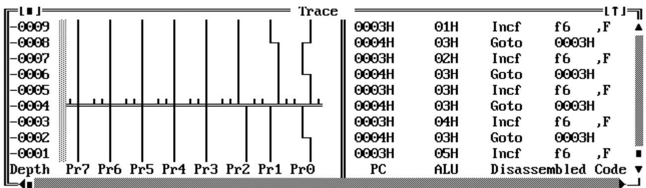
Moving the cursor in the trace listing can be controlled using arrow keys or the mouse. Move the cursor to the beginning of the line by the *Home* key and to the end of the line by the *End* key. To go to next or previous page of listing use the *PgDn* or *PgUp* keys. The *Ctrl-PgDn* or *Ctrl-PgUp* keys go to the beginning (to the youngest data) or top (to the oldest data) of the trace buffer.
